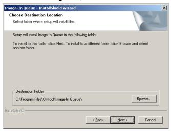
Note On 64 bit systems, the default destination folder is C:\Program Files (x86)\omtool\Image-In Queue.
