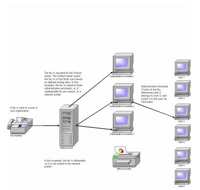
Figure 1-1. Example of routing rules
