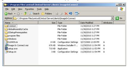
If you are installing Image-In Connect on a different system, ensure that proper access permissions have been set up for you to access the C:\Program Files\omtool\Omtool Server\clients\ImageInConnect directory. You can also copy the setup files to a shared network directory.
